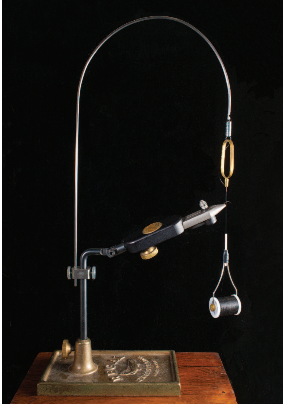
Above: A Regal vice with a Gallows Tool attached to it.
